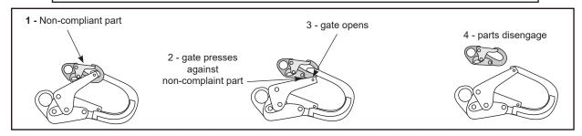
Using a connector that is undersized or irregular in shape (1) to connect a snap hook or carabiner could allow the connector to force open the gate of the snap hook or carabiner. When force is applied, the gate of the hook or carabiner presses against the non-compliant part (2) and forces open the gate (3). This allows the snap hook or carabiner to disengage (4) from the connection point.
