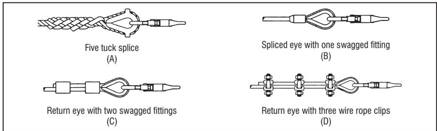
**IMPORTANT: Knots must not be used for load bearing end terminations. See ANSI Z359.1. Some knots reduce lifeline by strength 50% or more.**
